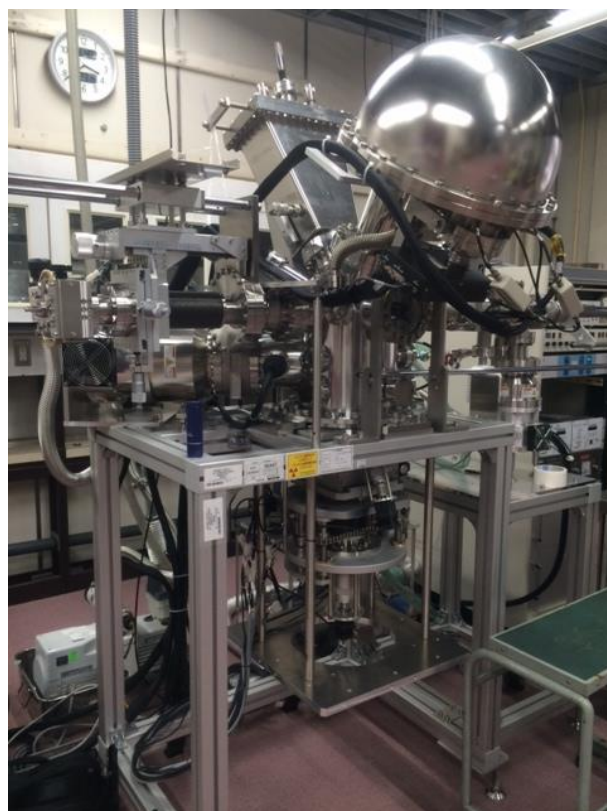
Fig.6: XPS equipment for surface analysis of Si sphere. (color online)
