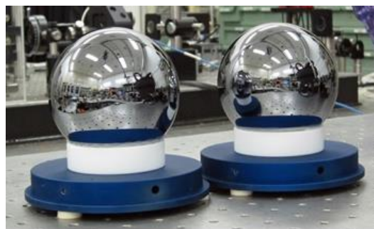
Fig.3: Isotopically enriched ^{28}\text{Si} single crystal produced by International Avogadro Coordination (IAC). (color online)
