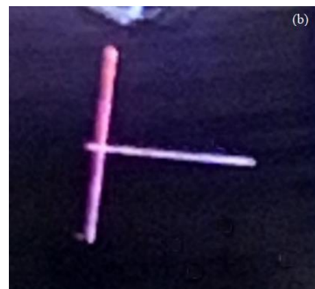
Fig.12: Markings on the ^{28}Si -enriched sphere. (a) on (100) lattice planes, (b) on (010) lattice plane. (color online)
